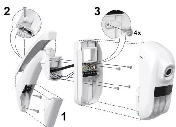
If wall bracket tamper is connected, tamper will automatically be detected by the camera. Tamper will follow recognition settings set in the panel.
