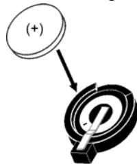
Figure 11: Changing the RTC's Battery
